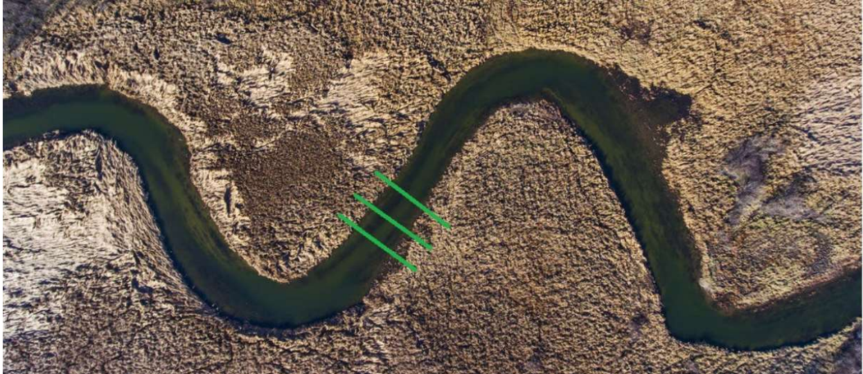
Figure 2. Measure width and depth cross sections at three locations in the stream reach where float time is recorded.
